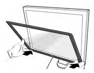
After mounting, press around the rim of the protective cover and leave it for at least 4 hours to allow the tape to adhere properly.
