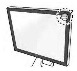
2. Use the suction cup to remove the protective cover from the LCD monitor.
