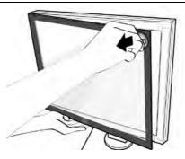
After removing the protective cover from the LCD monitor, push the tab to remove the suction cup from the protective cover. The dismounting procedure is then completed.
