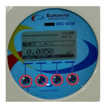
In the menu you can navigate up and down using the up and down arrows and 'OK' to enter the highlighted parameter. Pressing the '<<' will take you back to the previous screen.
