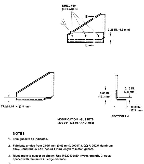
/4 Make sure the angle does not interfere with bend radius of gusset.
