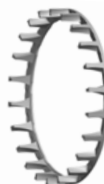
Fig. 9. Split, machined-brass, land-riding, finger-type cage.
