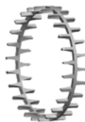
Fig. 7. One-piece, machined-brass, roller-riding, finger-type cage.
