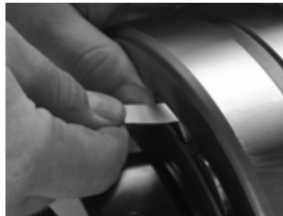
Fig. 14. Measure RIC before installation.
