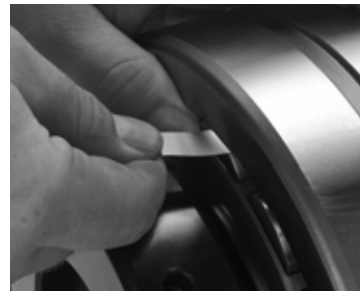
Fig. 18. Measure RIC before installation.
