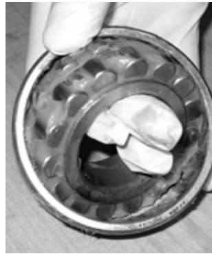
Fig. 21. Grease can easily be packed by hand.
