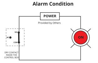
When the content inside one of the gas cylinder banks is depleted (low pressure), the dry contact switches from the Normally Closed (NC) position to Normally Open (NO) position. The electrical circuit is closed and the alarm device is actuated.
