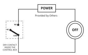
In this situation, both gas cylinder bank pressures are satisfactory (i.e. not empty). The dry contact inside the remote alarm box is in the Normally Closed position. The electrical circuit is open and the alarm device is NOT actuated.
