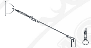
TRB 1/2"-4' Cable SUPPORT TRB 3/4"-4' Cable SUPPORT
