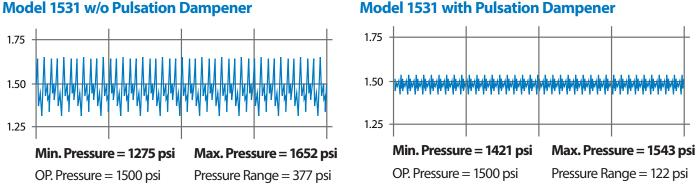
For best results, the dampeners should be mounted as close to the pump head as possible, preferably in a vertical position. Dampener should be charged at 60% of operating pressure.
