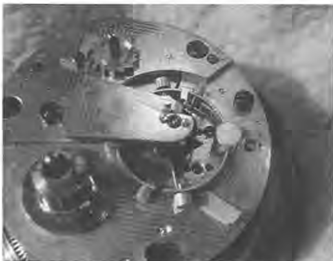
Photo 3. Later Kullberg balance from a chronometer by Hohwu of Amsterdam, ca. 1905. The affix is on the long balance arms.
