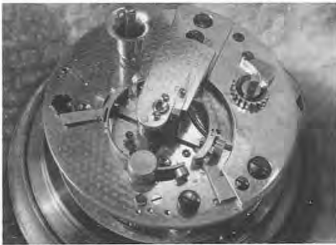
Photo 1. Poole's balance from a chronometer by John Poole of London, ca. 1858.
