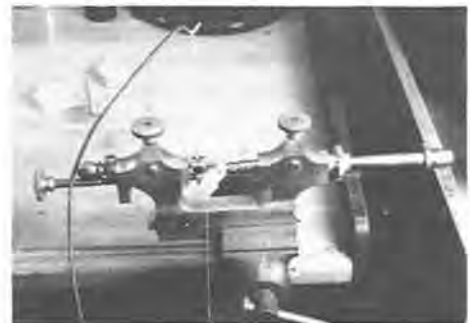
Figure 21. Jacot tool set up in the vise for use.
