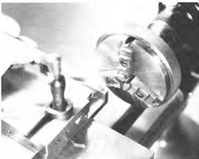
Figure 5. Watch this booby trap. Don't run the tool slide under the chuck jaws. Even worse, don't get a finger caught in this trap.
