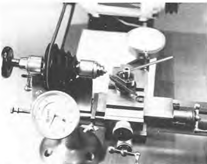
Figure 1. A Levin 3-deck slide on a Moseley lathe. Note the dial gauge attachments which also accommodate micrometer stops.
