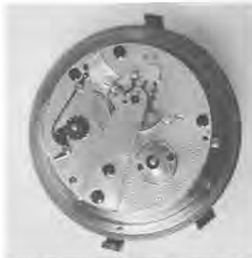
Photo 5. An experimental balance by Bliss and Creighton of New York, ca. 1845. The only structural innovation is that the balance rim is cut exactly 90 degrees from the balance spokes--a precursor to the Guillaume balance. This design would lessen the errors due to changes of centrifugal force.
