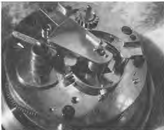
Photo 2. Early Kullberg balance from a chronometer by Pennington and Batty of Liverpool, ca. 1895. While difficult to see, the affix is on the short balance arms.
