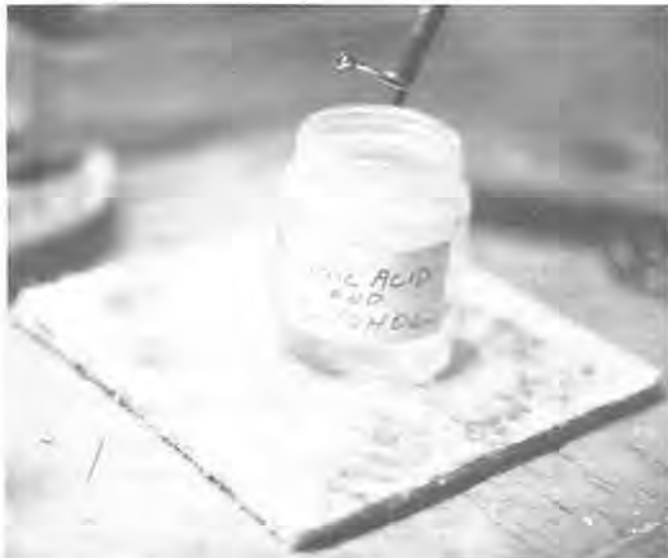
Figure 2. Boric acid and alcohol to prevent oxidation.
