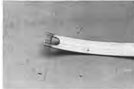
Figure 2. Alloy mainspring as it comes from the factory holding edge of hole.
