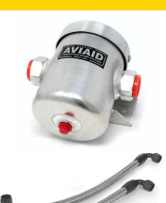
In addition to manufacturing a complete line of dry sump tanks that range in capacities from 1 to 3 gallons, Aviad makes a compact 1-quart tank that can be mounted near the engine. It measures 5" in diameter and also 5" in depth. There is internal reversing baffling and foam filler. It has two AN-12 female ports and a 3/8" NPT female drain plug bung.
