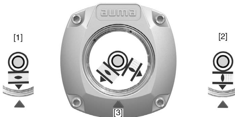
Figure 78: Mechanical position indicator
