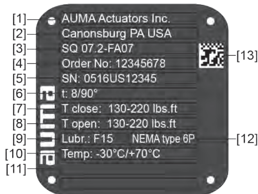
Figure 2: Actuator name plate (example)
