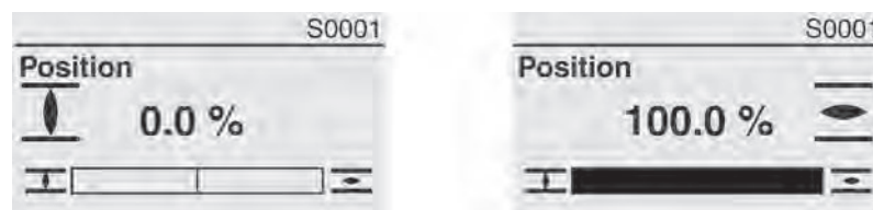
Figure 38: End position CLOSED/OPEN reached
