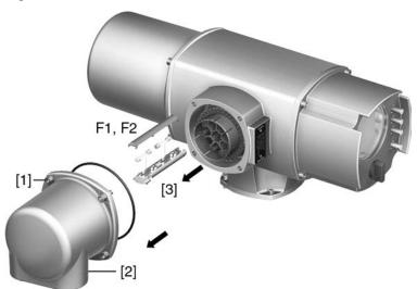
2. Pull fuse holder [3] out of pin carrier, open fuse cover and replace old fuses by new ones.
