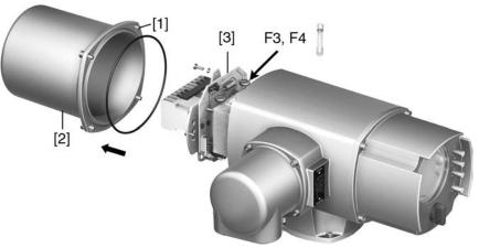
The power supply unit has measurement points (solder pins) allowing to perform a resistance (continuity) measurement:
