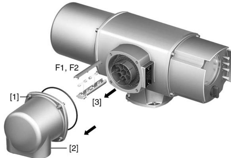
2. Pull fuse holder [3] out of pin carrier, open fuse cover and replace old fuses by new ones.
