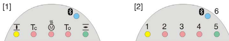
Figure 76: Arrangement and signification of indication lights
