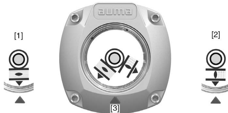
Figure 78: Mechanical position indicator
