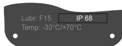
Figure 34: Name plate, example with enclosure protection IP68
