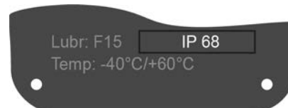
Figure 31: Name plate, example with enclosure protection IP68
