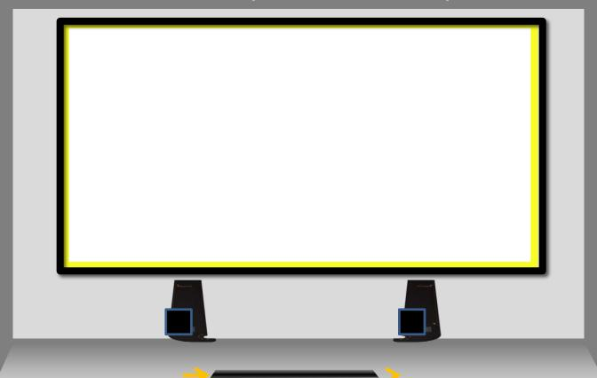
8. Mount the Fixed Frame Screen to the Wall using the yellow screen pattern as a guide.
