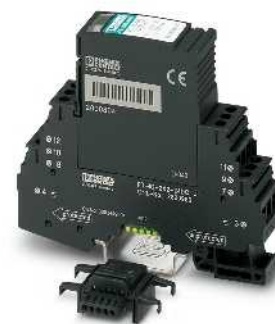
2 double wires (loops), floating, connection 9/10 grounded directly, e.g., for 4 ... 20 mA current loop
