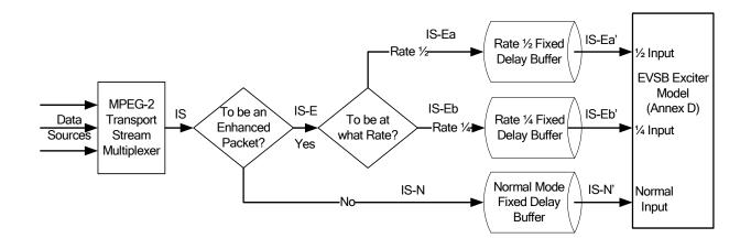
Figure 9.1 Head end reference model.
