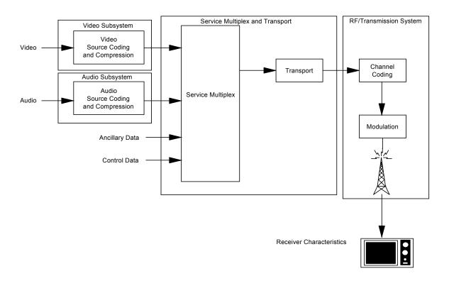
Figure 5.1 ITU-R digital terrestrial television broadcasting model.
