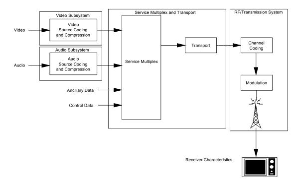
Figure 4.1 ITU-R digital terrestrial television broadcasting model.
