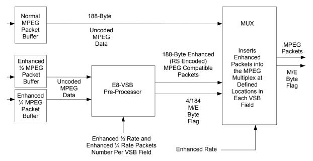
Figure 6.10 Main and Enhanced Mux Packet Processor.
