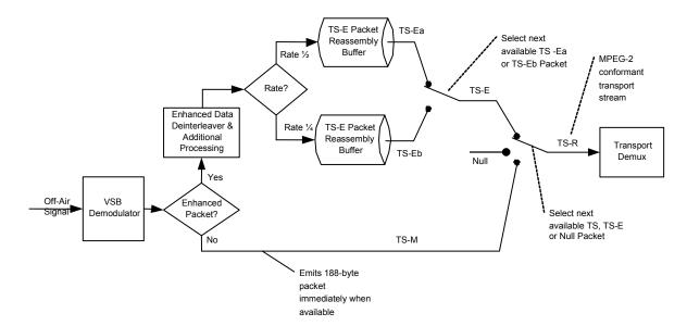
Figure 9.2 Reference receiver model.
