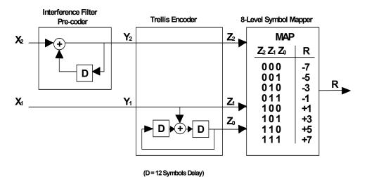
Figure 6.8 Main Service trellis encoder, precoder, and symbol mapper.
