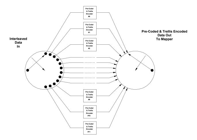
Figure 6.9 Trellis code interleaver.
