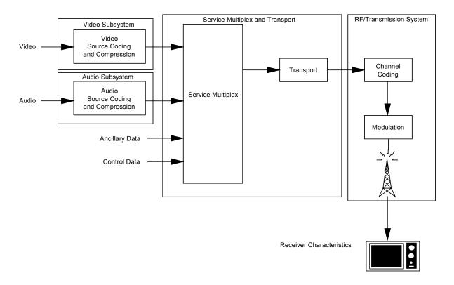
Figure 4.1 ITU-R digital terrestrial television broadcasting model.
