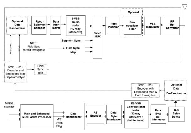
Figure 6.2 Main and Enhanced Service functional block diagram.
