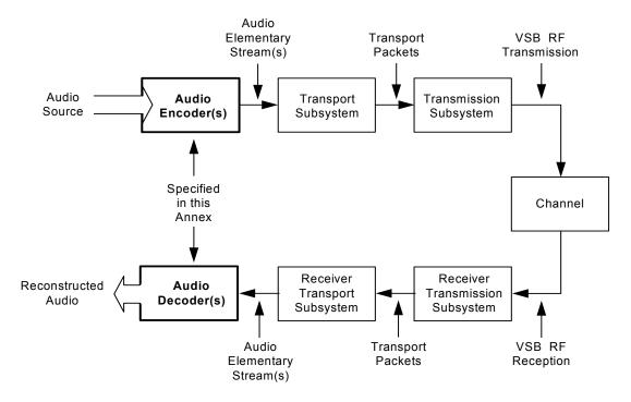
Figure 4.3 Audio subsystem in the digital television system.
