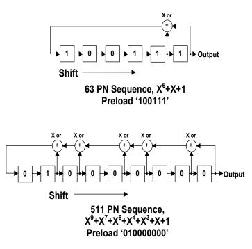
Figure 6.16 Field sync PN sequence generators.
