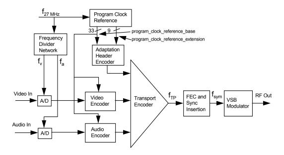
Figure 4.2 High level view of encoding equipment.
