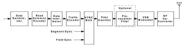
Figure 6.1 Main Service functional block diagram.
