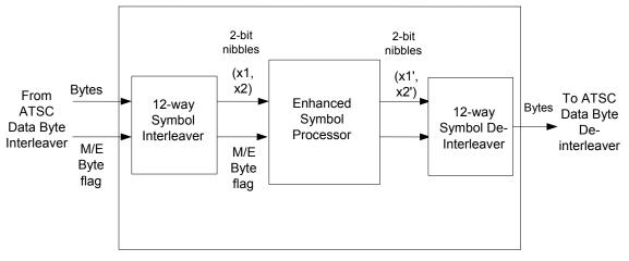
Figure 6.12 E8-VSB convolutional coder (12-way interleave/deinterleave).
