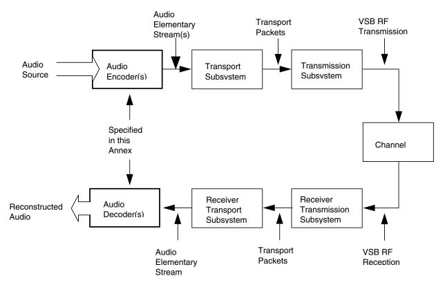
Figure 4.1 Audio subsystem in the digital television system.
