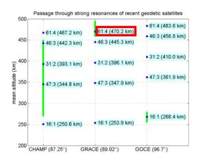
Figure 3. Passage through strong resonances of recent geodetic satellites. The altitude range, through which the particular satellite has already passed, is in green.
