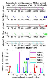
Figure 11. Histograms of node separation for orbits near the 61-day repeat orbit used in MOP1 of GOCE.
