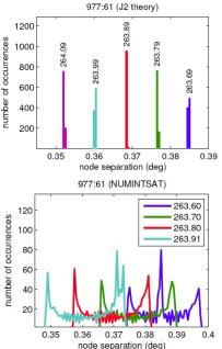
Figure 9. Histograms of the node separation for orbits computed with only J2 perturbation (upper graphs) and using all orbital perturbations (lower graphs).
