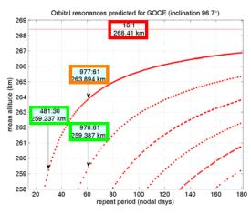
Figure 5. Resonance diagram for the GOCE satellite.
