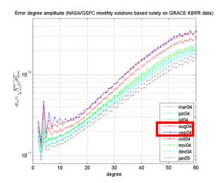
Figure 4. Error degree amplitude of monthly solutions from GRACE around the passage through the 61:4 resonance in August-September 2004.
