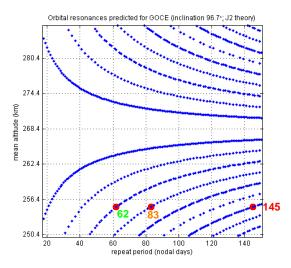
Figure 12. Resonance diagram for GOCE with the 145-day repeat orbit and the two other repeat orbits, which are the nearest in altitude.
