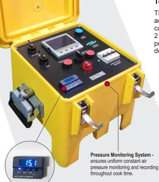
3 Phase Ammeter - built in to verify proper current draw to all phases to ensure even heat distribution, and to facilitate element diagnosis.
