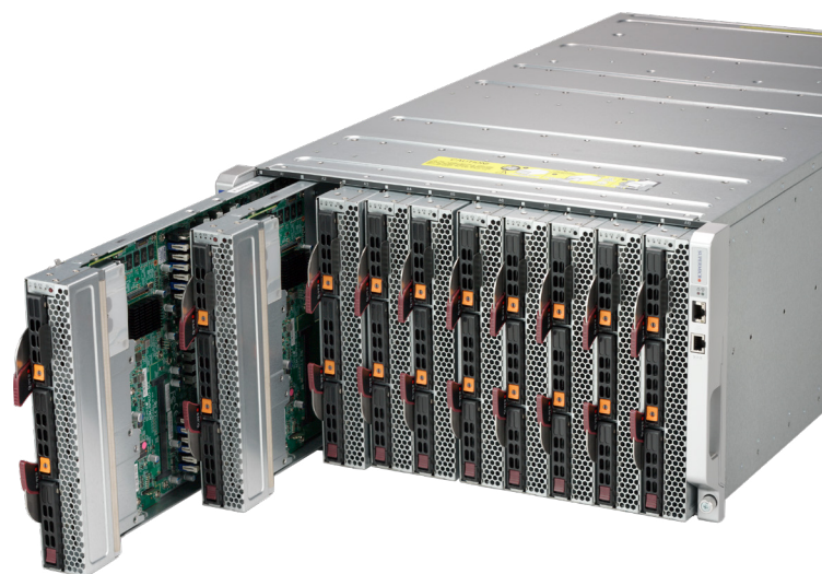
6U SuperBlade with 10 Blade Servers
