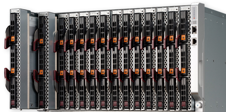
6U SuperBlade with 14 Blade Servers
