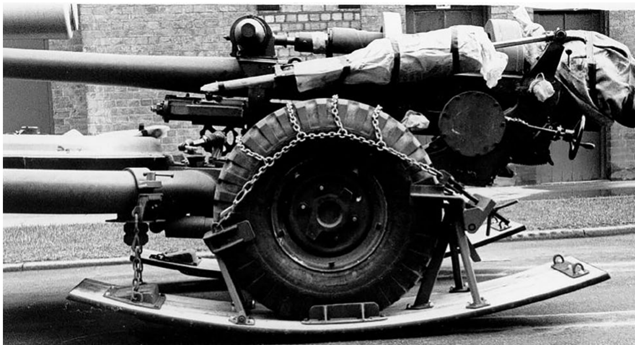
Skis are installed on an artillery piece during a 1987 Cold Regions Test Center Study on arctic mobility. These skis proved laborious to install, were ill-designed, and failed to significantly improve howitzer mobility. (Photo courtesy of the Cold Regions Test Center)
