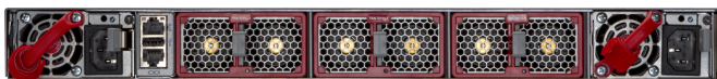
Arista 7280R3 1RU Rear View: Front to Rear airflow (red) AC Powered
