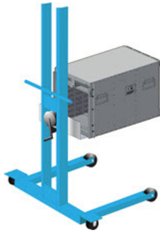
Figure 3-8 Lifting the chassis
