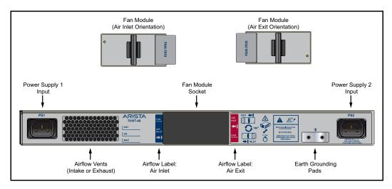
Figure 10: Orienting the Fan Module
