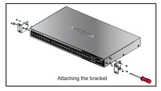
Figure 3: Attaching the Mounting Brackets to the Switch Chassis
