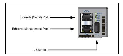
**Figure 9: Front Panel Ports**
