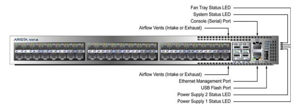
Figure 16: DCS-7010T-48 Front Panel
