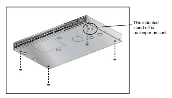
Figure 5: Attaching Rubber Pads to Bottom of Switch
