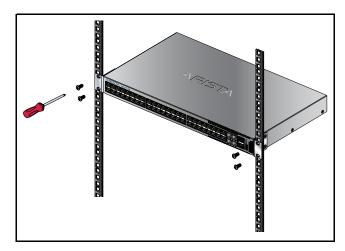
Figure 4: Inserting the Switch into the Rack
