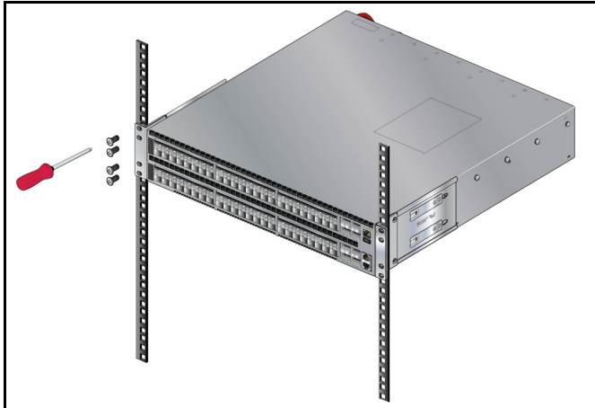
Figure 3-4: Inserting the Switch into the Rack
