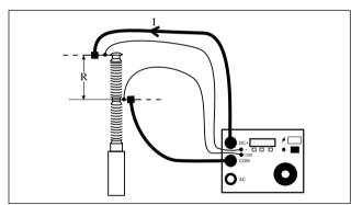
Measuring the resistance of a breaker
