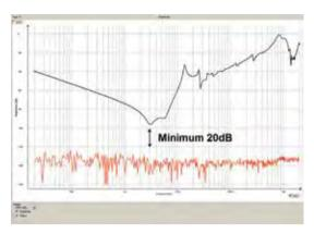
An example of a transformer measurement in comparison with the internal noise level in FRAX
