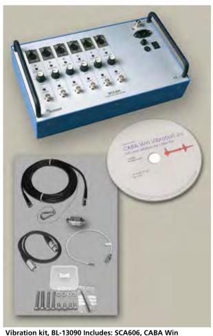
vibration software and one vibration channel
