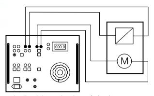
Testing the minimum trip voltage of a breaker.
