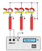
Basic circuit diagram of a phase identification
