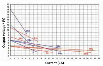
High current output - ODEN AT systems for 480 V, 60 Hz
