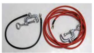
Current cables for SDRM201, the red cable is 3.0 m (9.8 ft) and the black one is 0.5 m (1.6 ft)
