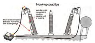
Solid connections using the C-clamps and the shortest braid method to connect the shield to ground makes it possible to eliminate connection problems and cable loops that otherwise affect the measurement.
