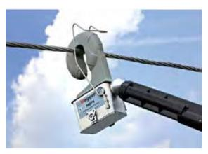
The Profilers are quickly installed at any point on the distribution line and are mountable to many readily available clamp sticks.
