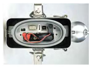
Easy plug-in access allows for quick data retrieval via RS-232 and USB cable ports. The battery compartment is specifically designed for simple removal and installation.
