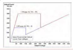
$<sup>^{\</sup>rm 2}$  PowerVTM output current varies depending on the voltage setting on the 150 Volt range, see curve.
