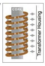
The SFRA method is based on comparisons between measured curves where variations are detected. One SFRA test consists of multiple sweeps and reveals if the transformer's mechanical or electrical integrity has been jeopardized.
