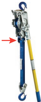
Convertible Version With bracket that eliminates need for third hook
