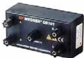
6311-077 CB101, 5 kV calibration box
