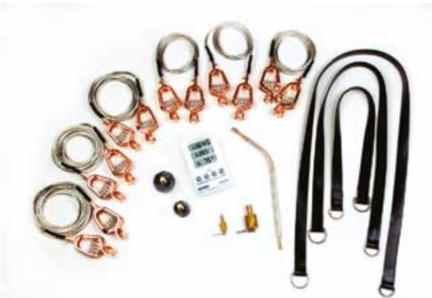
The optional accessory kit, C/N 670501 includes mini bushing tap connectors, hot collar straps, temperature/humidity meter, .75" bushing tap connector, 1" bushing tap connector, "J" probe bushing tap connector, 3-ft non-insulating shorting leads, 6-ft non-insulating shorting leads.
