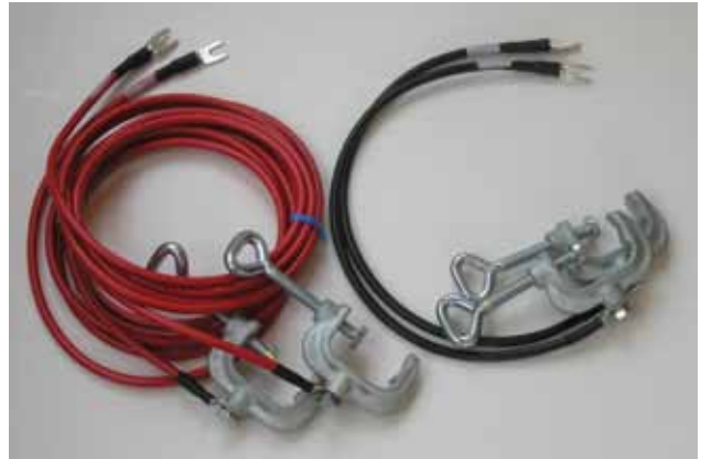
The red current cables are 3.0 m (9.8 ft) and the black ones are 0.5 m (1.6 ft).
