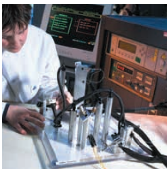
▲ AUTOMATIC CONTINUITY & INSULATION RESISTANCE TEST
