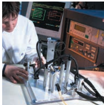
▲ AUTOMATIC CONTINUITY & INSULATION RESISTANCE TEST
