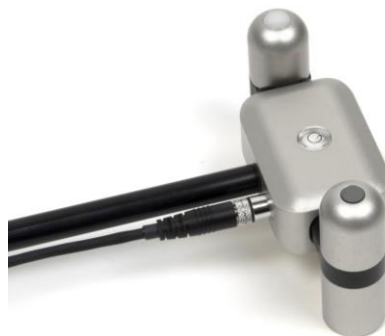
Cable connectors are attached directly to the head.
