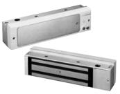
The M490DE Series Delayed Egress Magnetic Lock is a self-contained unit, designed to meet the NFPA 101 Life Safety Code. It is an easy-to-install, cost-effective solution to life safety and security applications. Delayed egress is triggered by an internal "plunger switch," to cause a 15- or 30-second delay and audible sound. Onboard contacts are provided for reset and legal release.
