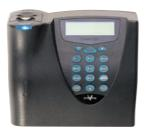
The V-Station-A authenticates users with dual-factor authentication, combining the power of biometrics with PIN numbers. PIN numbers can no longer be borrowed or given out to others, since they have to match an employee finger scan.
