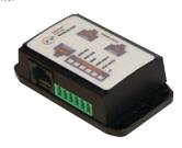
The TZ Centurion Port Link provides dynamic and cost-effective security, sensing and power expansion of the TZ Centurion System. These interconnect modules enable networking of TZ locking and environmental-monitoring devices.
