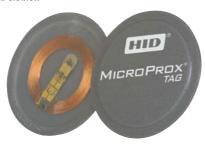
The MicroProx Tag provides the convenience of HID's Proximity technology in a small disk-shaped transponder. Simply attach the adhesive-backed tag to any nonmetallic card or device and you instantly have a Proximity card.
