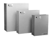
Recommended where an interface with a fire-alarm system or battery backup is needed. The BPS linear power supply delivers more current than PSPs or PMs, and all BPS models are UL Class 2 Listed, allowing for wire runs without the use of conduit from power supply to door. The BPSH series operates with 220 V AC.
