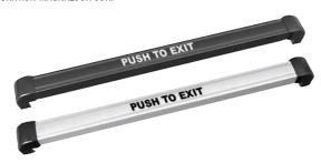
The Touch Sense Bar is for use on magnetically locked, non-fire-rated doors. Touching the bar, even through light gloves or clothing, trips an electronic sensor which releases the lock. For indoor use only, the TSB-3 can be installed on metal, aluminum, or wood frame doors of all types. Meets "no special tools or knowledge" code requirements.
