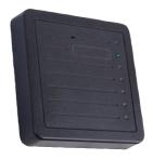
The D8223 Prox Pro Reader provides Wiegand protocol interface capability in a black, easily mounted, weather-resistant enclosure. The reader is designed to fit a vertically mounted, U.S.-standard, single-gang switch box for easy installation. It is field-adjustable through a selectable jumper setting so that it can be mounted directly to metal with minimal impact on its read-range performance.
