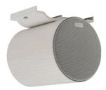
The LBC 3432/02 is a powerful 20 W sound projector intended for speech and music reproduction in indoor and outdoor applications. The sturdy, aluminum enclosure is finished in off-white. It has provisions for both cable loop-through connection and the mounting of a line or loudspeaker supervision board. The sound projector is suitable for use in voice alarm systems.
