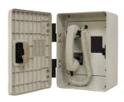
GAI-Tronics' industrial telephones are designed for those applications where standard telephones are not environmentally suitable. The auto-dial telephones are programmed to automatically dial when the handset is taken off the hook. The phones have a detachable programming keypad, preventing unauthorized tampering of the preprogrammed phone number.
