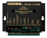
The C-1000B allows single-line phones or phone systems to share a phone line with one or two doorboxes or paging amplifiers. In addition, the C-1000B provides two touch-tone-controlled relays to operate door strikes or gate openers. The C-1000B provides two touch-tone-controlled relays to operate door strikes or gate openers and provides doorbox triggered CCTV camera switching.
