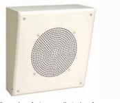
The MB8TSQ and MB8TSL speakers feature an all-steel surface-mounted enclosure with an 8 in. cone loudspeaker and multitap 4-watt 70V/25V transformer. The MB8TSQ is suitable for ceiling or wall mounting. The MB8TSL is designed primarily for wall mounting and its face is angled downward by 12.5 degrees.
