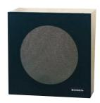
Bogen's wall baffle is ruggedly constructed of 3/8 in. particle board with reinforced corners. It is finished in simulated walnut and will house any of Bogen's 8 in. speakers. A sloping front panel provides enhanced downward dispersion. Hardware for mounting a speaker to the baffle included.
