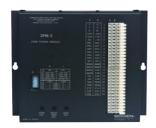
The ZPM3 allows for economical one- or two-way paging (with TBA 15 Talk-Back Amplifier) to be directed into any of up to three different paging areas. Zones can be grouped together so that more than one zone is paged at the same time. All areas can also be paged at once. Zone selection can be made using DTMF tones or pulse dialing.
