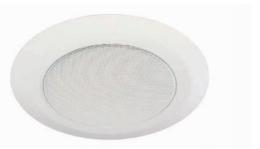
The Quam C10FX/H70/2WS is a complete loudspeaker assembly, with 8 in. speaker, transformer, designer two-piece grill with a fine-mesh center insert, 10 in. diameter, durable, paintable white baked epoxy hybrid finish.
