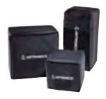
Air Plugs are used to fill in cable openings in the raised floor or any gaps where airflow needs to be blocked. Air Plugs are soft, compressible and safe to use around all types of cable, including fiber optic cable. Mighty Mo Air Plugs are made from the fireproof material Sandel. All plugs have a height of 5 in..
