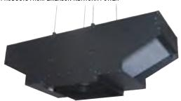
Th Liebert XDO overhead cooling module mounts directly above the cold aisle, requiring no floor space. It draws in hot air from the hot aisle, then discharges cool air into the cold aisle where the equipment air inlets are located. Liebert XD refrigerant-based cooling modules work as a system to support the hot aisle/cold aisle approach to cooling high-heat-density data centers. The modules provide focused rack cooling, enhancing a room precision cooling unit, such as a Liebert DS system.
