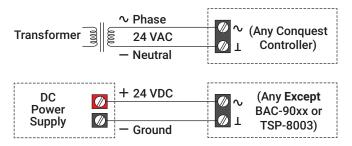
Illustration: 24 VAC and VDC Power Connections
