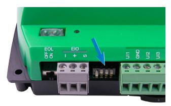
Illustration: Expansion Module Address Switches
