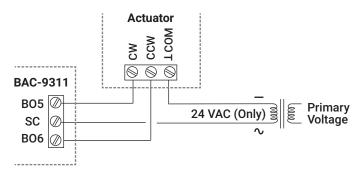
**Illustration: Remote Actuator Wiring**
