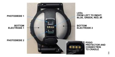
Figure 4. Connections and Buttons–Bottom of Watch
