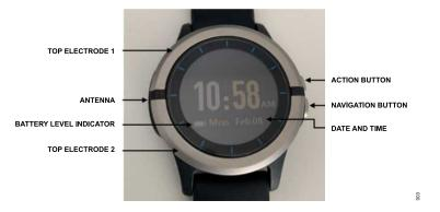
Figure 3. Connections and Buttons–Top of Watch
