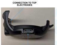
MICRO USB CONNECTION FOR EXTERNAL ELECTRODES
