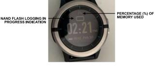
Figure 20. NAND Flash Logging Indicator with Percentage of Memory Used
