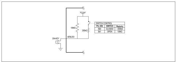
Figure 4. nENLDO Pullup Resistor Configuration
