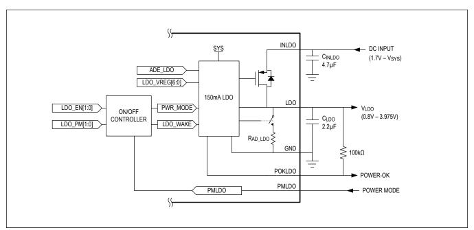
Figure 13. LDO Simplified Block Diagram
