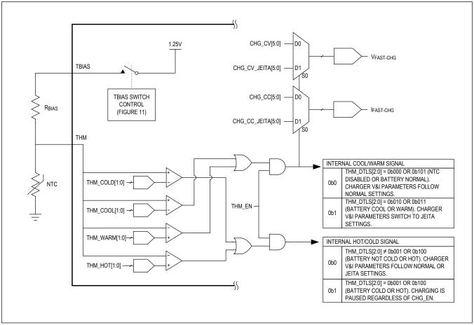
Figure 9. Thermistor Logic Functional Diagram
