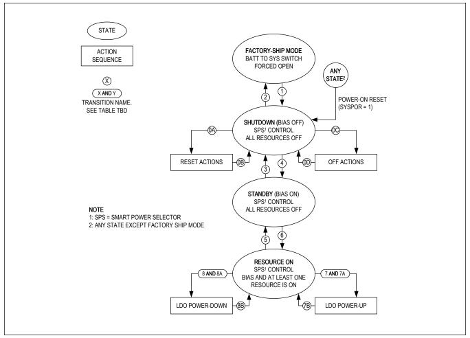
Figure 1. On/Off Controller State Machine
