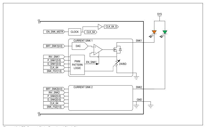
Figure 16. LED Current Sinks Functional Block Diagram
