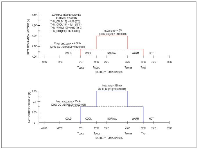
Figure 10. Safe-Charging Profile Example
