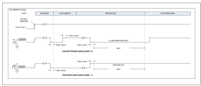
Figure 3. nENLDO Dual-Functionality Timing Diagram
