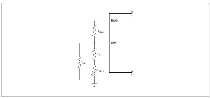
Figure 12. Thermistor Circuit with Adjusting Series and Parallel Resistors
