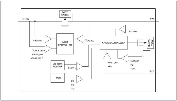
Figure 6. Charger Simplified Control Loops
