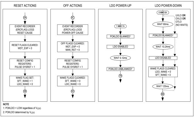
Figure 2. On/Off Controller Action Sequences
