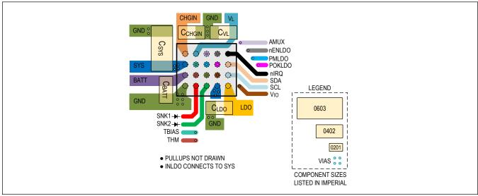
Figure 15. PCB Top-Metal and Component Layout Example
