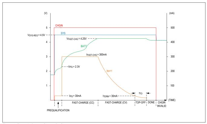
Figure 8. Example Battery Charge Profile
