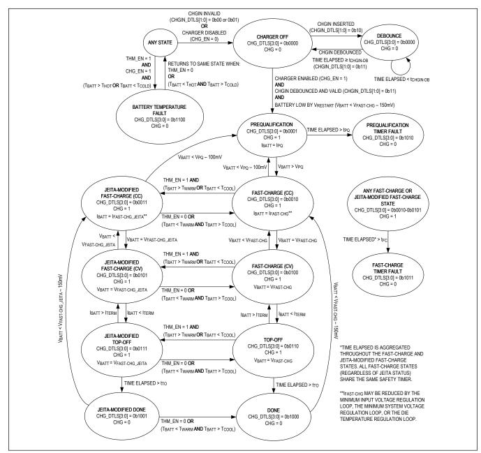
Figure 7. Charger State Diagram
