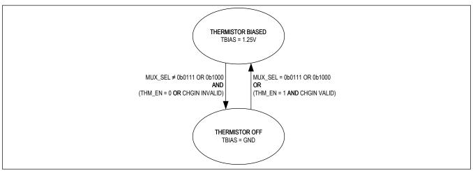
Figure 11. Thermistor Bias State Diagram
