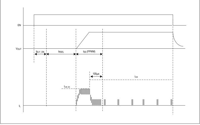
Figure 1. Startup Waveform
