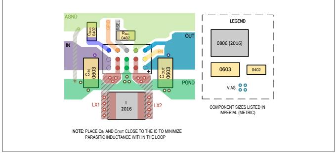
Figure 4. PCB Layout Example (WLP)
