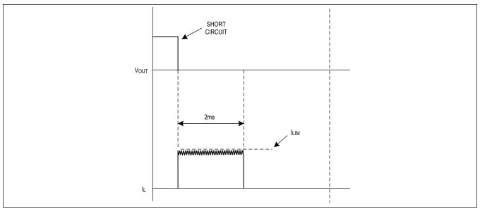
Figure 2. Short-Circuit Waveform
