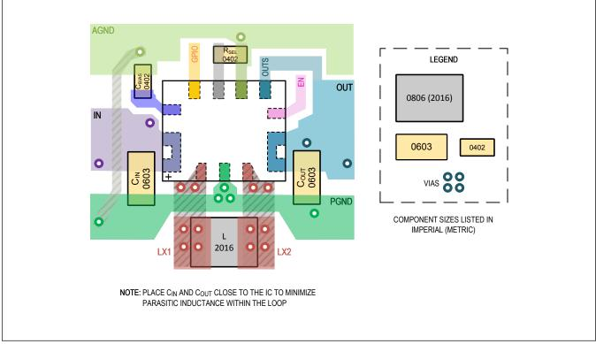
Figure 5. PCB Layout Example (FC2QFN)
