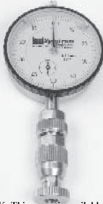
Type K: This gauge is available with a resolution of 0.01mm, or 0.001 inches.
