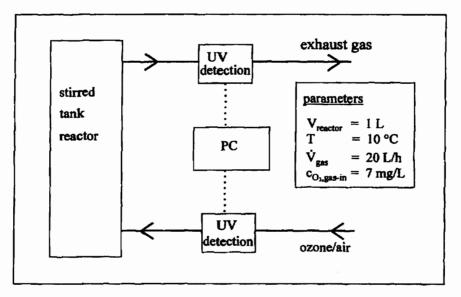
Fig. 1: Apparatus scheme for ozonation.
