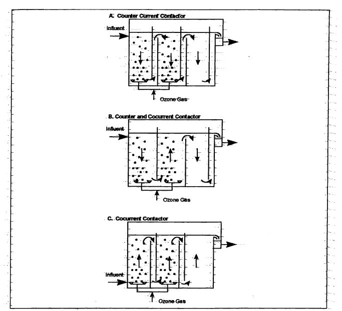
Figure 3-7. Ozone Bubble Contactor
