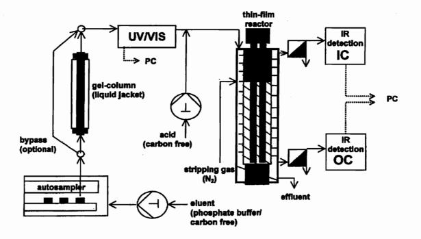
Fig. 2. LC-DOC/UV system (schematical).
