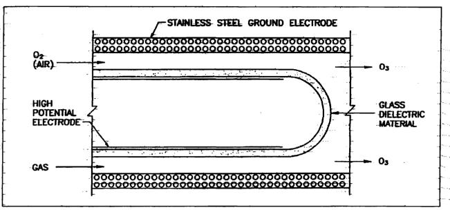
flowing around the stainless steel ground electrodes. The tubes are arranged in either a horizontal or vertical configuration in a stainless steel shell, with cooling water circulating through the shell.
