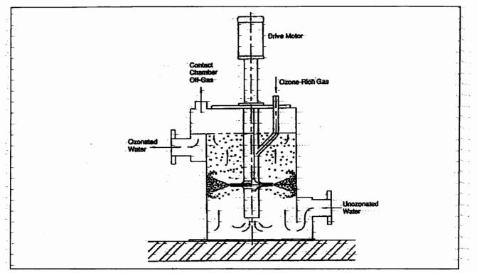
Figure 3-9. Turbine Mixer Ozone Contactor
