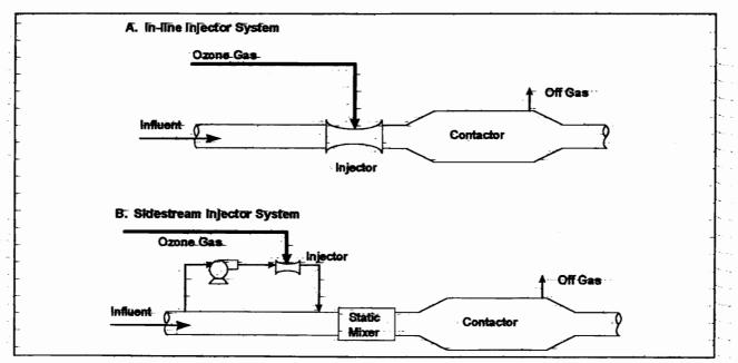
Figure 3-8. Sidestream Ozone Injection System
