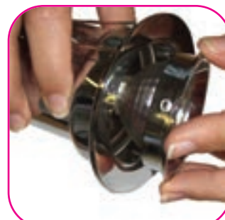
Step 5 Push twist ring into lamp housing and twist ring clockwise
