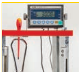
INSULATION ADHESION TEST
