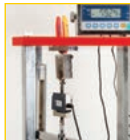
INSULATION ADHESION TEST
