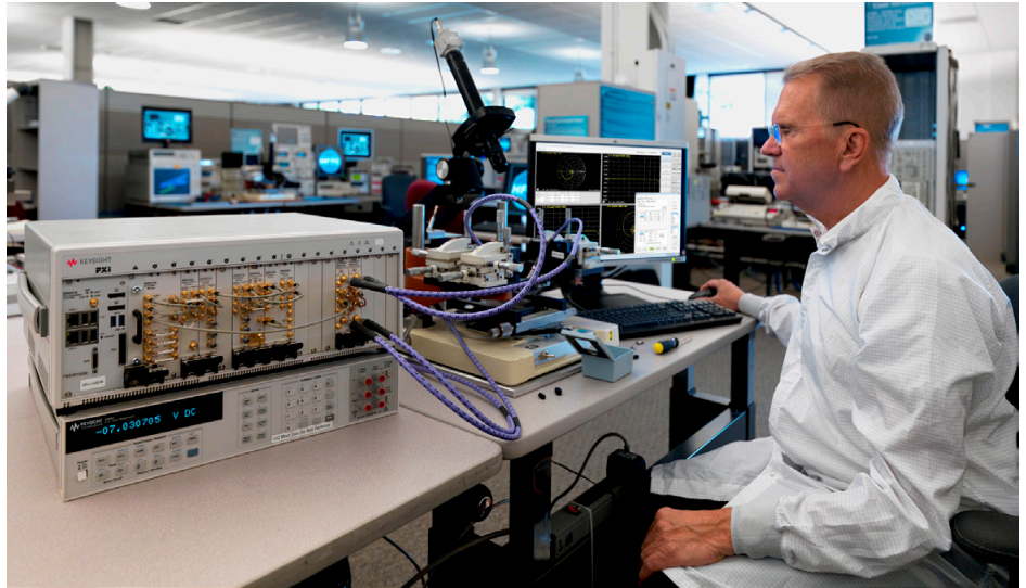
Using Keysight's M937xA PXIe vector network analyzer, M9381A PXIe vector signal generator and M9391A PXIe vector signal analyzer with measurement application software for power amplifier test.
