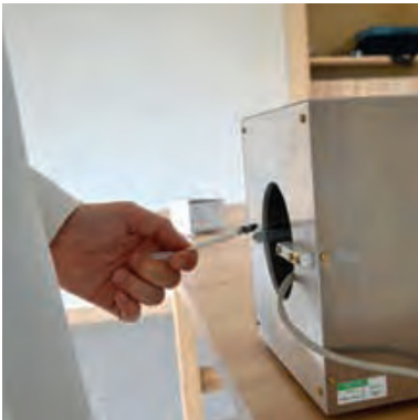
▲ FIGURE 2: This item's initial magnetic state is being measured using a three-axis probe, whilst protected by the magnetic shield
