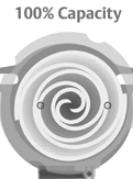
capacity for better efficiency and humidity control. Based on demand, the modulation ring is activated, sealing the bypass ports and instantly shifting capacity to 100%. Take advantage of "shift on the fly" stage changing (no stopping and starting required like other two-stage compressors).
