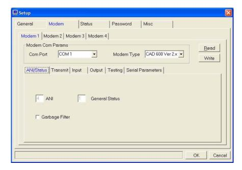
**Note:** Prior to writing to the modem, the RX Input must either be quieted or disconnected. If there is noise present at the RX Input during modem programming, it may interfere with programming and result in EEPROM corruption.
