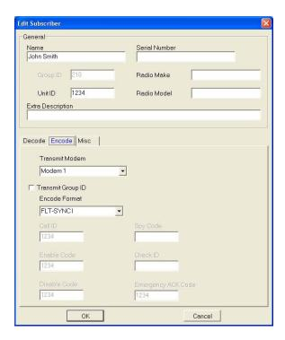
**Transmit Modem:** This should be set to the desired modem that was set up in the CAD Setup > Modem.
