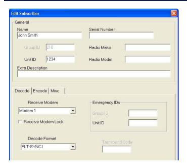
Name: This is the alias for the Unit ID that will be displayed when a Unit ID is decoded.
