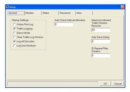
Online Print Log: If checked the CAD software will output all incoming traffic to a printer connected to LPT1.
