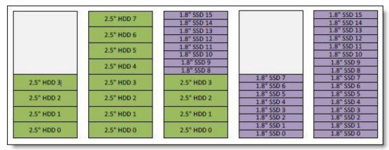
Figure 6. Internal drive configurations
