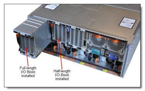
Figure 12. Optional I/O Books that are installed (x3850 X6 shown)
