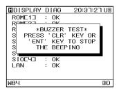
After self-diagnosis has been performed for the screen, the entire screen is highlighted repeatedly such as black to white, white to black. Check if some dots are omitted.
